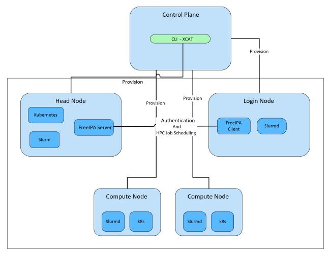
Omnia performs bare metal configuration to enable AI/HPC workloads. It uses Ansible playbooks to perform installations and configurations. iDRAC is supported for provisioning bare metal servers. Omnia installs xCAT to enable provisioning of clusters via PXE in different ways:
